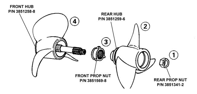
Figure 1. DuoProp® Propeller Installation
