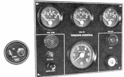
The instrument panel is provided with a key switch, rev counter, temperature gauge, oil pressure gauge and voltmeter, warning lamp for connection of glow plugs, reostated switch for instrument panel light. Cable harness, 7 m (23 ft.) in length, with plug-in contact already fitted, for connection to engine and instrument. Control lamp and switch for drive lift and 7 m (23 ft.) electric cable harness with plug-in contact are also supplied.
