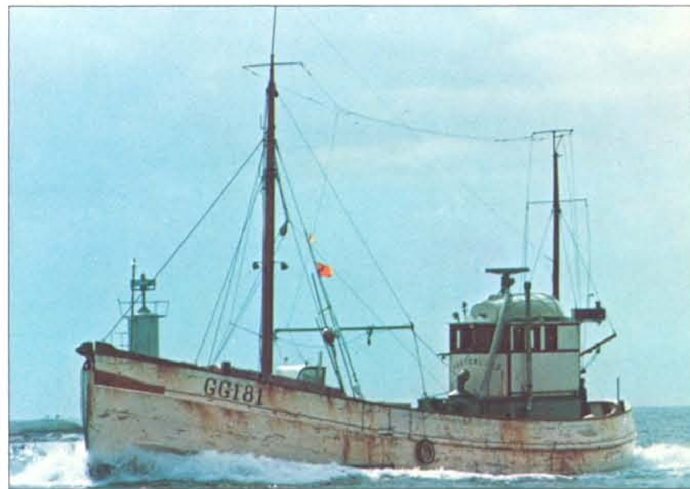
“VÄSTERLAND” GG 181 Höno, Sweden 76 ton trawler powered by Volvo Penta TAMD 120 A Reverse gear: TWD MG 514. Ratio: 5.16:1 Propeller: 3-blade variable pitch Speed: 10 knots
