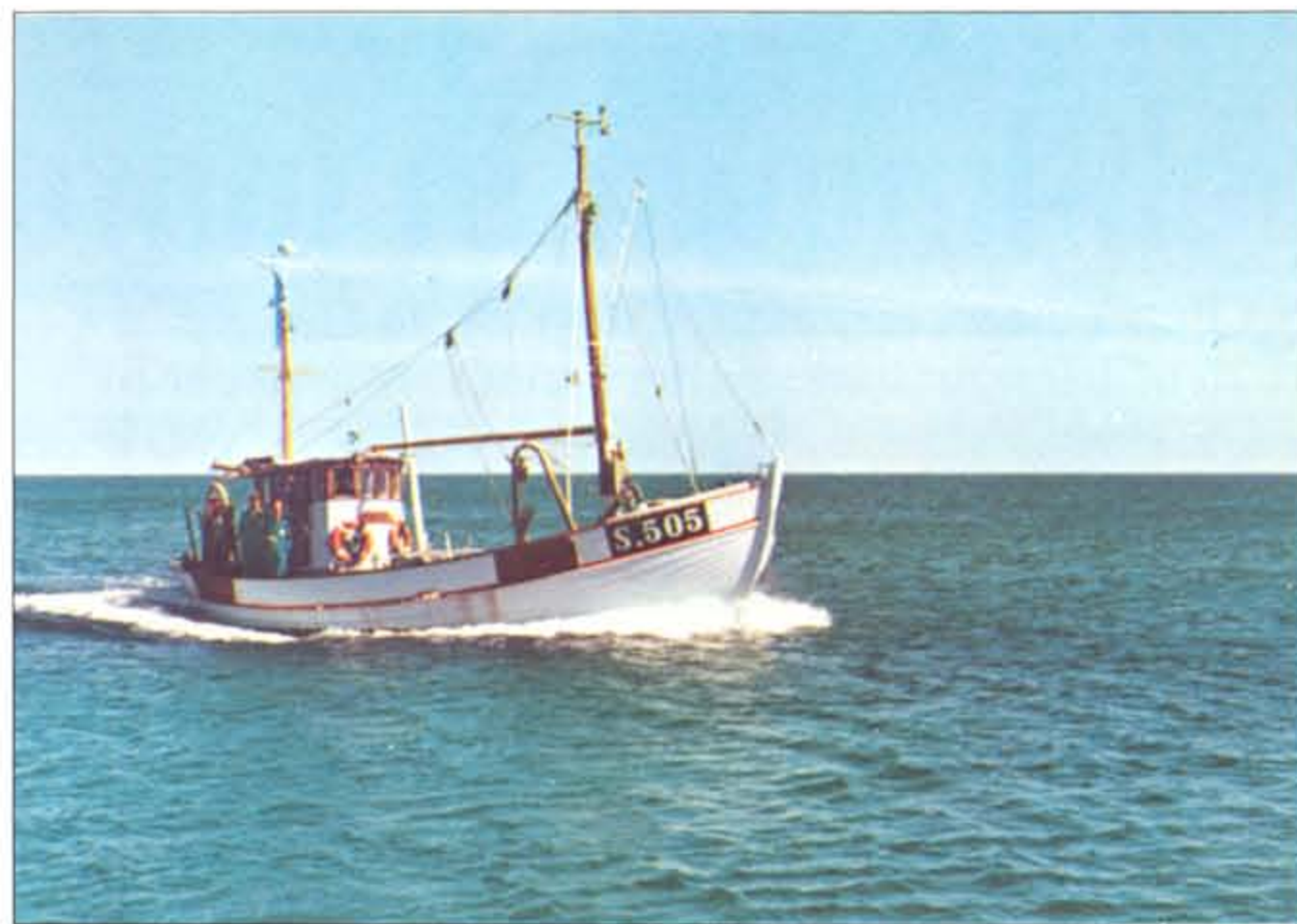
“ANNA MARIE” S505 Aalbeck, Denmark 13 ton trawler powered by Volvo Penta TMD 70 B Reverse gear: TWD 506. Ratio 4.5:1 Propeller: Hundested 1200 mm fixed, adjustable Speed: 9.0 knots
