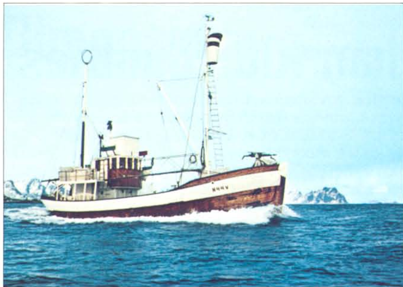
“DÖNNÖY” N 44 V Lofoten, Norway 63-ft, combined trawler and whale catcher powered by Volvo Penta TAMD 120 A Reverse gear: TWD 514. Ratio: 5.16:1 Propeller: Heimdal 1,600 mm fixed, adjustable Speed: 10.5 knots
