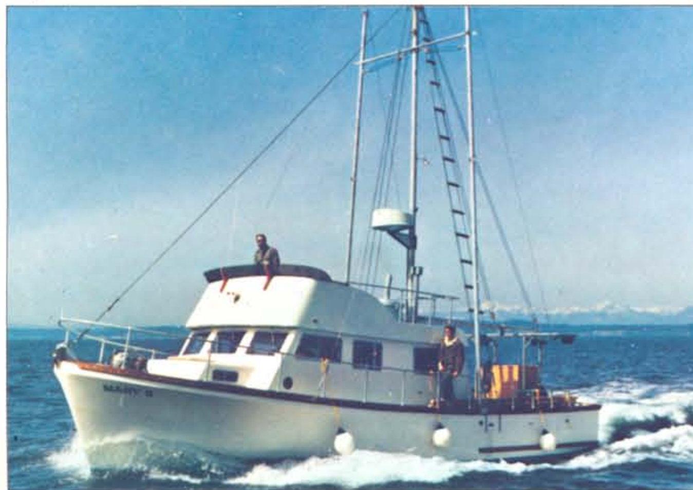
“MARY E” Ketchikan, Alaska 29 ton trawler powered by Volvo Penta TMD 70 Reverse gear: TWD MG 506. Ratio: 2.96:1 Propeller: 3-blade 810 mm Speed: 9 knots
