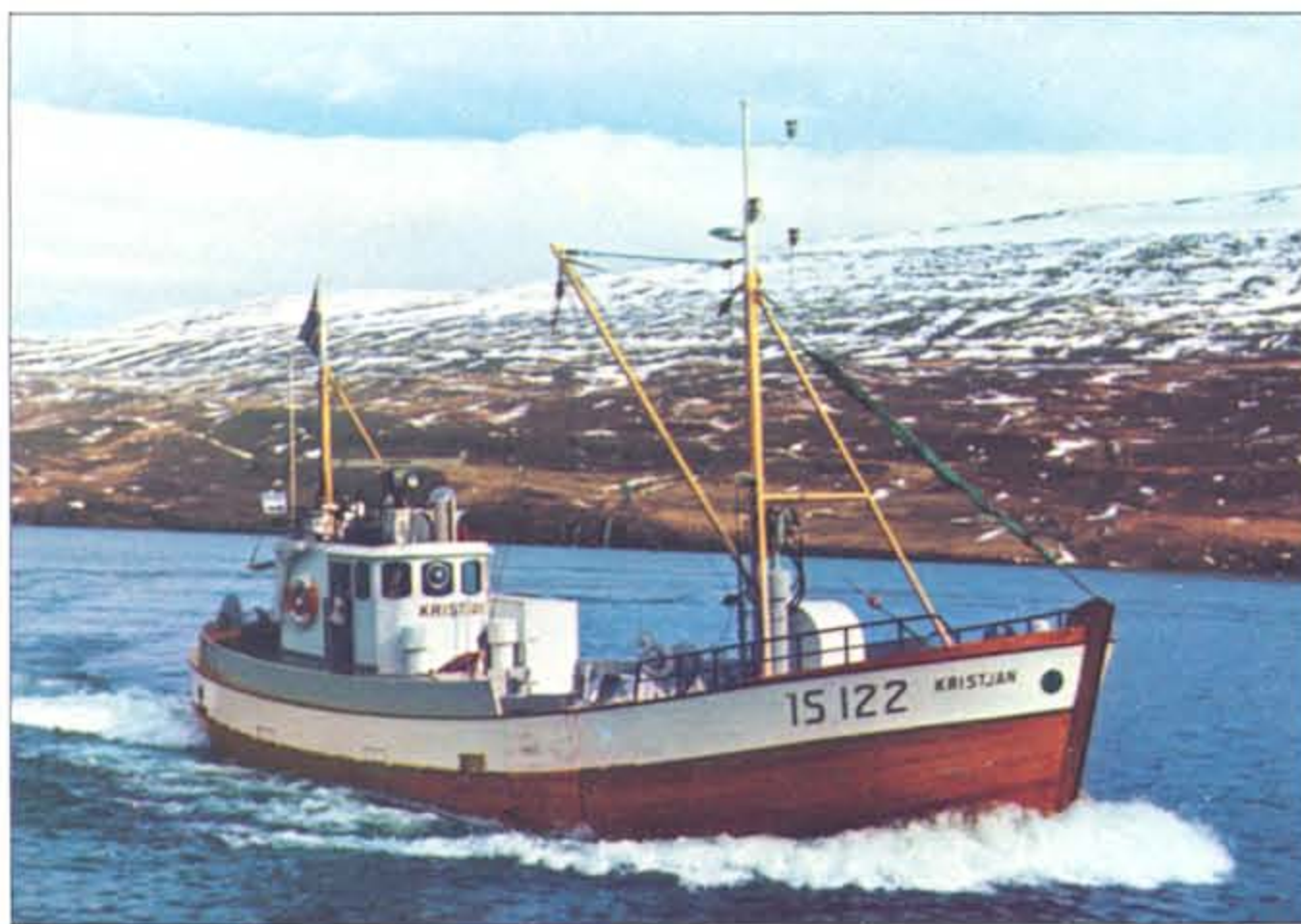
“KRISTJAN” 15122 Akureyri, Iceland 30 ton combined line and netter powered by Volvo Penta TMD 120 A Reverse gear: TWD 514. Ratio: 3.5:1 Propeller: Federal 4-blade 1160 mm Speed: 10.5 knots
