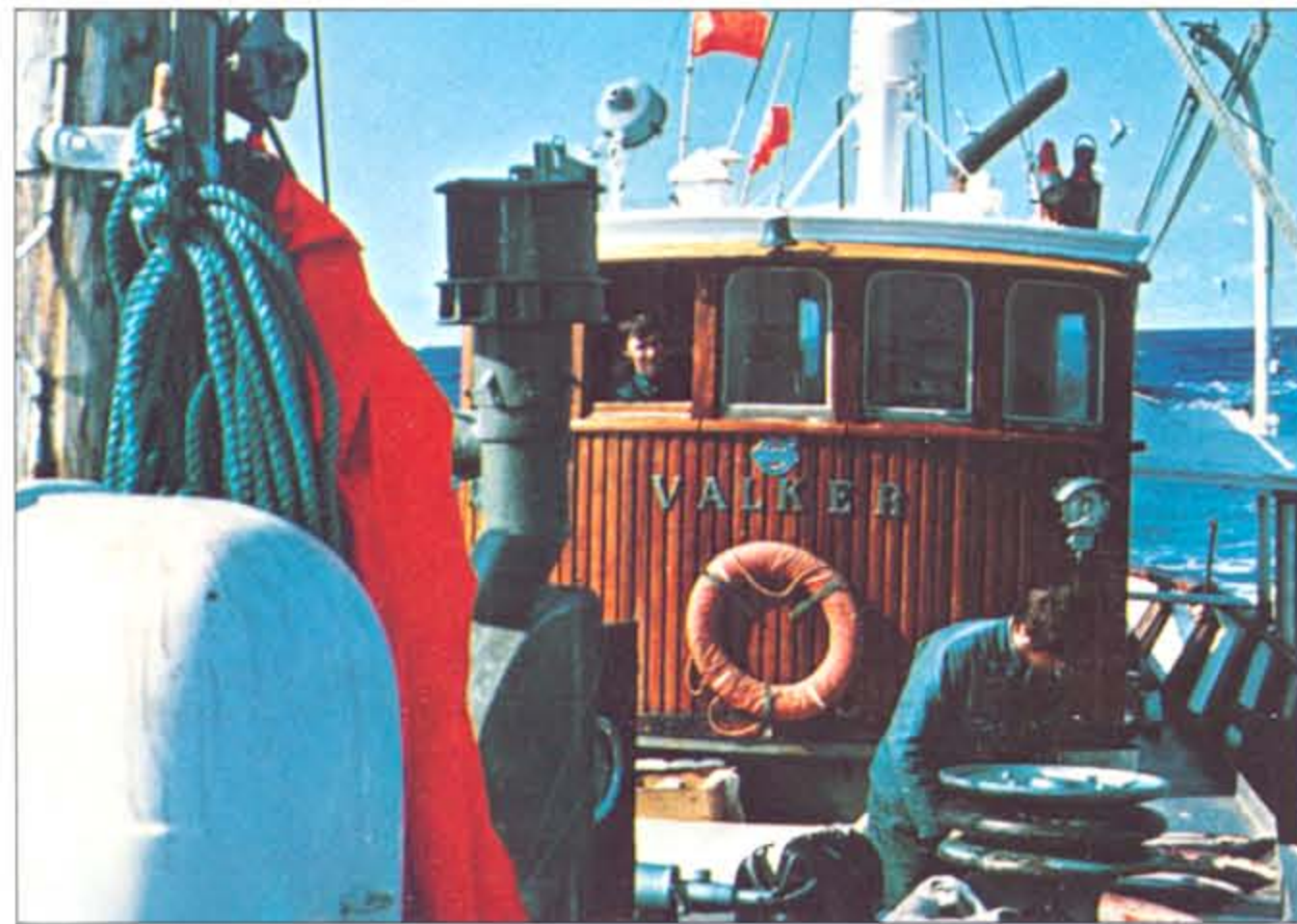
“VALKER” N 116 A Bleik Andöya, Norway 57-ft, combined line and netter powered by Volvo Penta TMD 120 A Reverse gear: TWD 514. Ratio: 4.5:1 Propeller: Heimdal 1350 mm fixed, adjustable Speed: 9.5 knots
