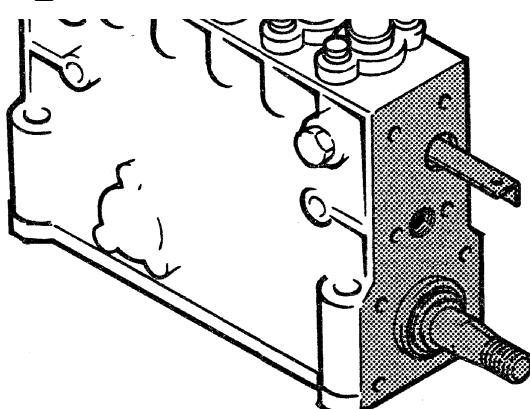
Clean the pump face and camshaft end carefully.
