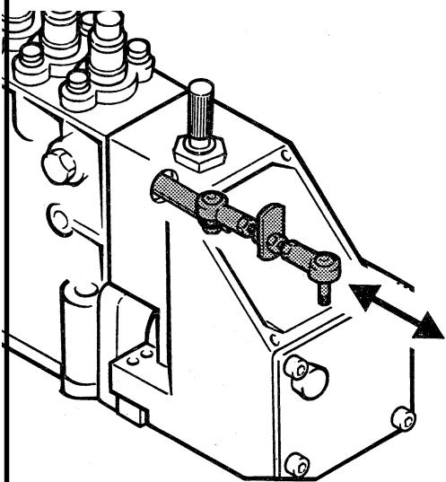
Check that the control rod can move freely over the full stroke and does not jam in any position.
