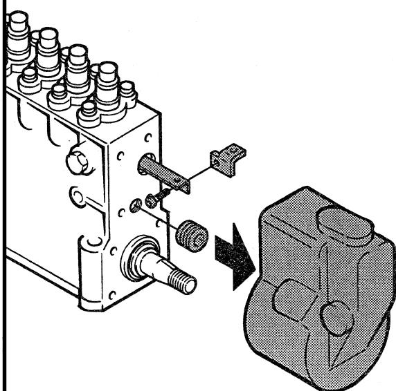
Observe great care when dismantling the stop lever so that the control rod is not bent.
