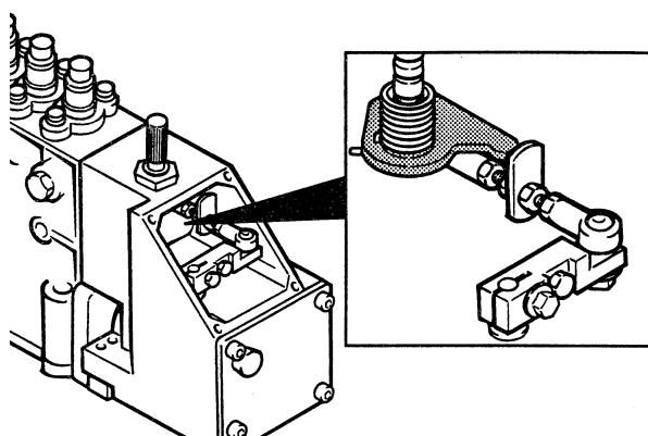
Check that the stop plate on the governor's stop lever makes proper contact with the stop plate on the ball joint and that the control rod can be moved back to the 0-position.
