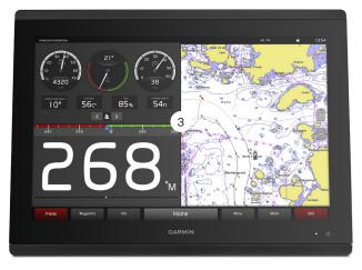
Fully customizable layouts and views. All active functions and alarms are displayed in the status bar (1). Information overlays can be placed anywhere on the display (2). Information can be divided up to six times with split screen function (3).
