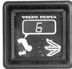
The trim angle is indicated by five green diode lamps plus a digital display. A continuous red light indicates when the drive is in the "beach" sector. The red light flashes when the drive is in the "tilt" position.
