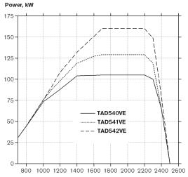
Engine speed, rpm
