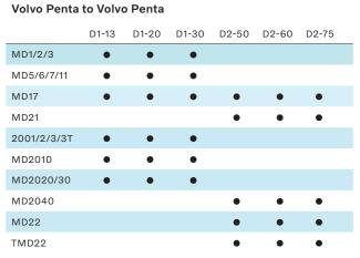
Note: For above installations, the existing reverse gear must be replaced.
